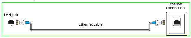
• Connect an Ethernet cable (not provided) to the LAN jack on your TV and to your Ethernet connection.
